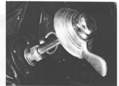
Reassembly of the steering, washer, cap screw and light switch tube.
